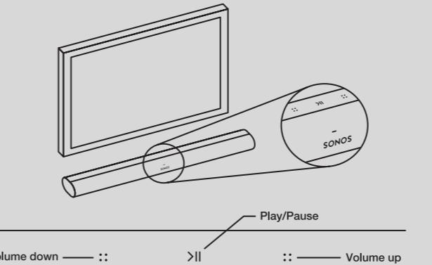
**NOTE:** Make sure the touch controls on Arc are facing up when you position it.
