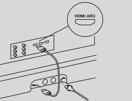
**NOTE:** The optical adapter in the box is only needed if your TV doesn't have an ARC port. (Dolby Atmos won't be supported.)
